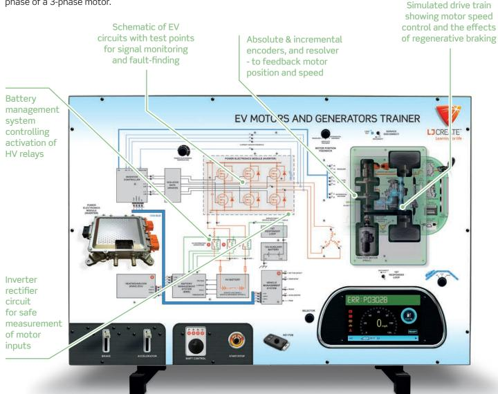
Test points with reduced voltages for safe measurement
