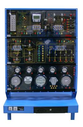
The ConsuLab MP-1918-1 is a CAN Bus Multiplex trainer that communicates in J-1939 protocol. Digital and analog inputs and outputs can be activated. Analog signals can be displayed using the J-1939 display. The trainer utilizes the "Moduponent®" design feature which allows unlimited expansion capabilities. This unit is equipped with an integrated electronic fault box containing 12 faults.
