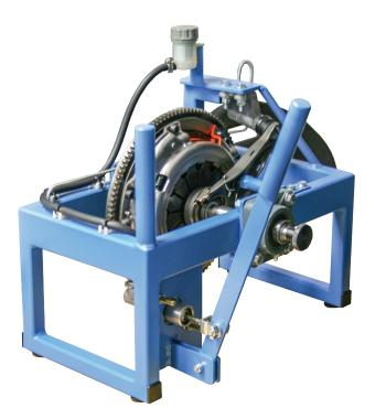
As an instructor, have you struggled to demonstrate how a clutch system works to your students? The new EC-1120 is a working system of actual, all new components so that students can visualize the actual operation and make your life easier as an instructor.
