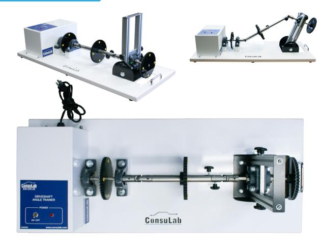
The ConsuLab EM-200-28 is designed to help demonstrate and simplify the complex acceleration and deceleration phenomenon that occurs in revolving universal joints and drive shafts operating at various angles. Even when the input driveshaft rotates at constant speed the output driveshaft maintains a variable speed depending on the angle between them, which causes vibrations and wear over time. The higher the angle between the shafts the more amplified the effect is.
